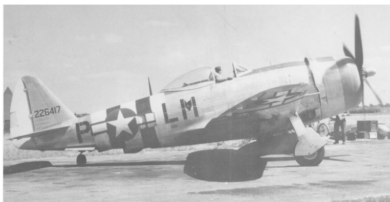
Major Lucian A. Dade, Jr., 62d Fighter Squadron, flew this P-47D-25 with a bubble canopy during June 1944. Shown is Tail Number 42-26417, painted with the D-Day paint scheme. Dade later commanded the 56th Fighter Group. He also commanded Luke's 3600th Maintenance and Supply Group in the mid-1950s.
